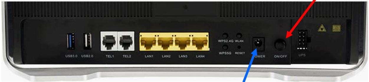
2. Or you can unplug the power cord which is located to the left of the ON/OFF Button. Wait 1 minute and re-plug in to restart the ONT.
